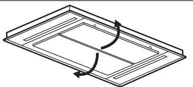
2. Press the handle of the mounting clip on the filter panel underneath the hood (1).
